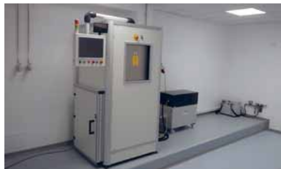
Figure 2: The X-ray irradiator installed at TIFPA in December 2016, with the power generator on its side and the water cooling system on the background.
