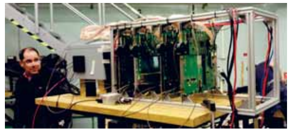
Figure 1: pCT apparatus at The Svedberg Laboratory (Uppsala, Sweden) beam line : tracker (green boards) and calorimeter(gray box).
