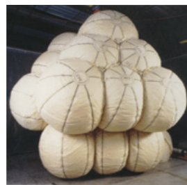
Airbag per lander Mars Pathfinder, Jet Propulsion Laboratory, NASA 1996.
