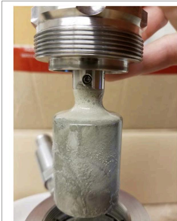
**FIGURE 5 |** The pressurization/depressurization of the samples yielded a substantial volume of foam on top of the inner cylinder of the pressure cell. Picture taken after removing the inner cylinder from the pressure cell.
