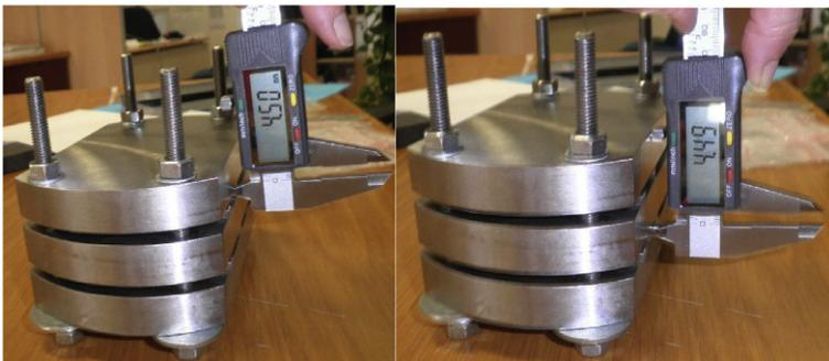
Fig. 7 Compression set test—details of the deflection.
