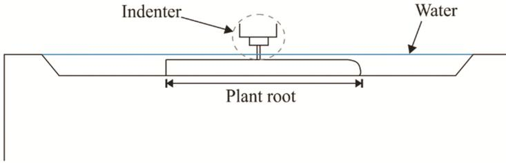
**Fig. 2.** Schematic of the setup used for testing along the root at different distances from the tip.
