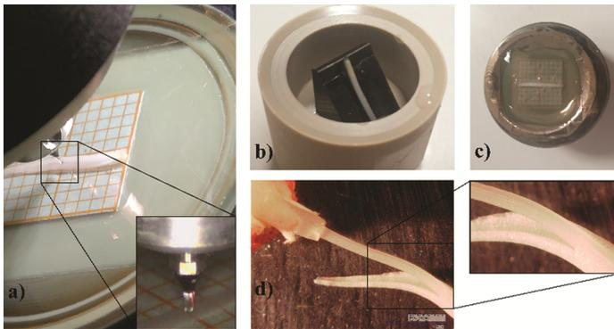
**Fig. 1.** View of a nanoindentation experiment. (a) A nanoindentation test. The zoom shows the tip of the indentation system; (b) and (c) a sample holder used to test mechanical properties of root tissues near to the cap, and in outer and inner areas, respectively; (d) separation procedure of the outer wall from the inner core.
