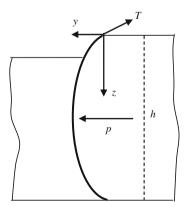
Fig. 81.1 Scheme of the textile barrage (*side view*)
