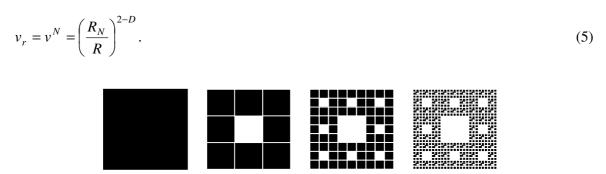
Figure 2. The Sierpinski carpet (D=1.89) at different levels of observation; it corresponds to the cross section of a deterministic hierarchical bar in which the white zones represent the soft matrix, and the black ones are the hard inclusions.
