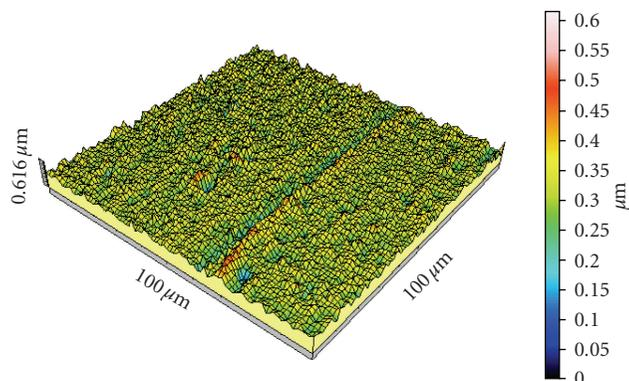
FIGURE 2: Glass: surface of glass without any superficial treatment.
