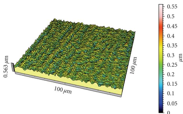
FIGURE 3: Plexiglass: surface of plexiglass without any superficial treatment.
