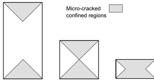
Fig. 1. Micro-cracked confined regions for friction tests
