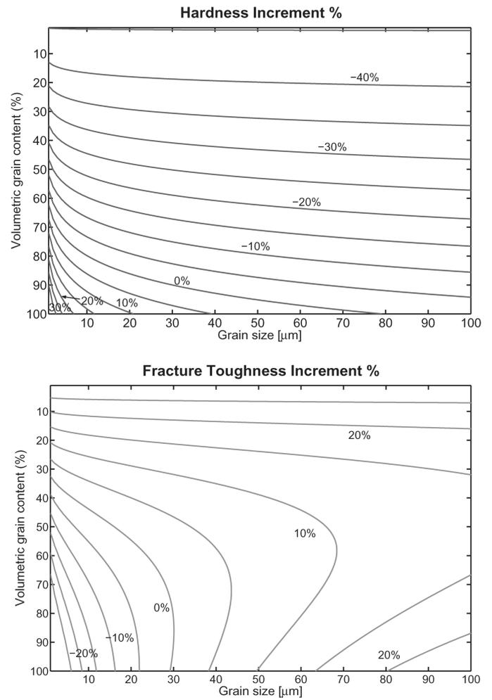
**Fig. 3 Iso-hardness lines (top) and iso-toughness lines (bottom). Numbers along the curves indicate hardness and fracture toughness increments %.**
