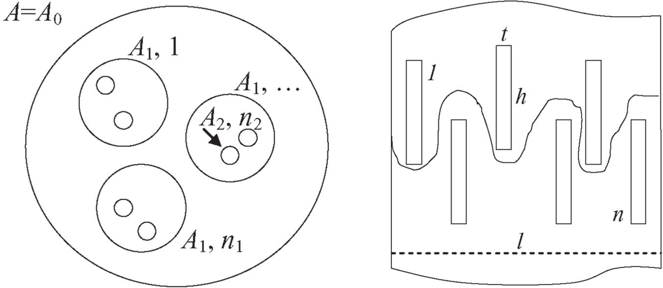
**Fig. 1** The cross-section of a hierarchical bar (left) and the lateral view of the crack surface (right) corresponding to the toughening mechanism.
