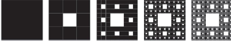
**Fig. 2** The Sierpinski carpet ( $D=1.89$ ) at different level of observation; it corresponds to a deterministic hierarchical bar in which the empty space is the soft matrix, and the complementary zones are the hard inclusions.
