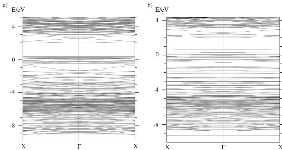
**Figure 7.** Two band structures of defective AlN nanosheets containing a single F centre per doubly extended unit cell of armchair-type (a) and zigzag-type (b) NS chiralities.
