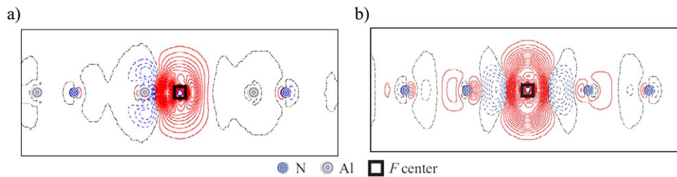
**Figure 6.** 2D difference electron density maps  $\Delta\rho(\mathbf{r})$  (see explanations given in figure 4) projected onto the section planes across AlN NS containing a single F centre per doubly extended unit cell with a structure of (a) armchair-type (figure 2(a)) or (b) zigzag-type (figure 2(b)) NS chiralities. For graphical details, see explanations given in figure 4.
