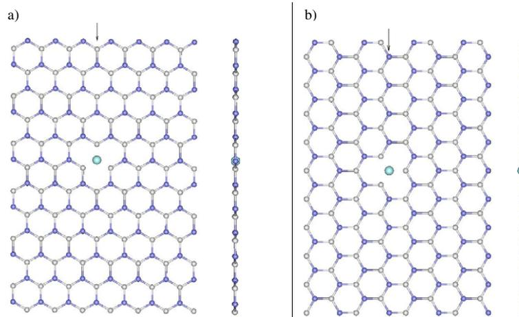
**Figure 2.** Projections of AlN nanosheets containing a single F centre for wrapping up to 1 nm-thick nanotubes (shown in figure 3) along the axes of NSs and across them for: (a) armchair-type and (b) zigzag-type chiralities. Arrows show section planes for 2D difference electron density plots presented in figure 6. For graphical details, see explanations given in figure 1.
