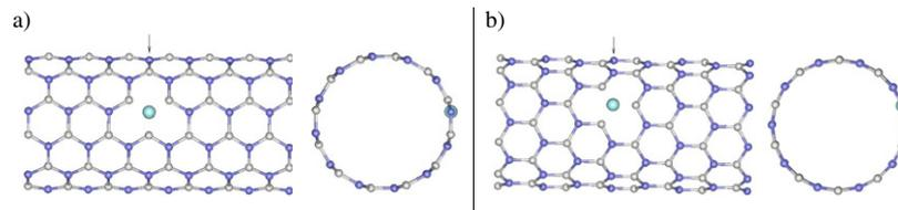
**Figure 3.** Projections of 1 nm-thick defective AlN NTs along the axes of nanotubes and across them for: (a) armchair-type and (b) zigzag-type chiralities. Arrows show section planes for 2D difference electron density plots shown in figure 8. For graphical details, see explanations given in figure 1.
