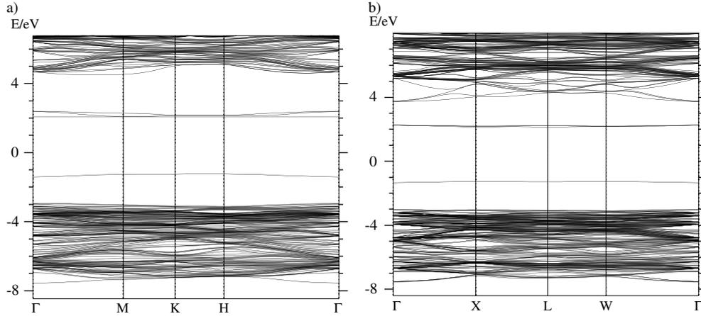
**Figure 5.** Two band structures of defective AlN bulk containing a single F centre per cell in both a  $3 \times 3 \times 3$  supercell of a wurtzite crystal (a) and a  $4 \times 4 \times 4$  supercell of a zinc-blende lattice (b).
