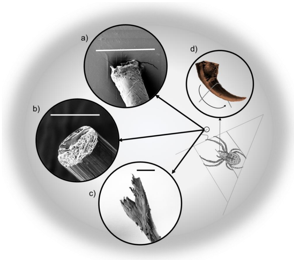
Fig. S4. Cross-sections of the silk, carbon and Kevlar® fibres cut by spiders. The interaction of the spider and its webs (artificial and natural) has revealed that these animals can cut a) silk lines, b) carbon fibres, and c) Kevlar® fibres (SEM images of the fibres' cross-sections after the spider cutting). Scale bars 6 \mu\text{m} . d) Hypothesized movement of the fangs to cut the fibres.
