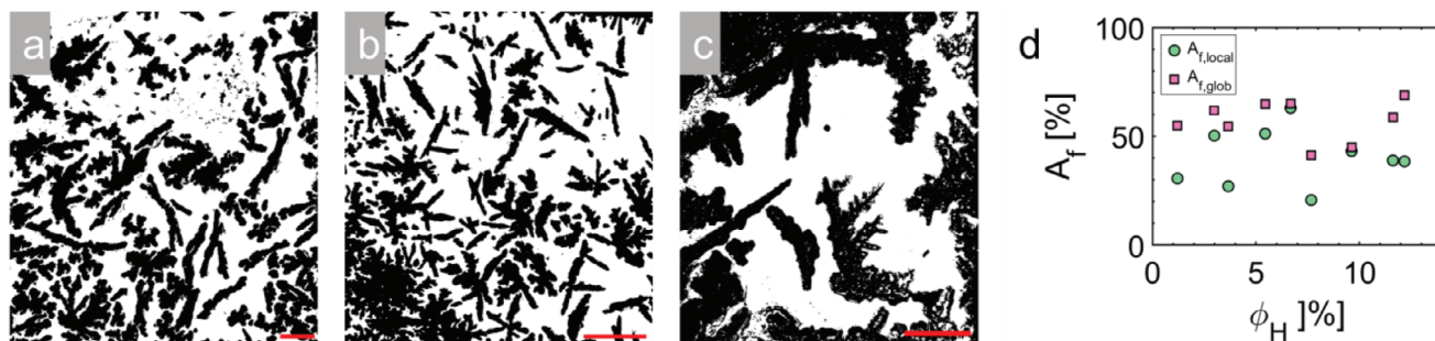
Figure 9. From a) to c), the frost on the patterned area (global) of Surface_15 \times 20, Surface_30 \times 40, and Surface_10 \times 20, respectively. d) A_{f, \text{glob}} and A_{f, \text{local}} as \phi_H varies. Scale bars 2 mm.
