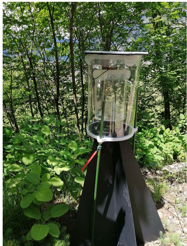
Fig. 1 Vibrotrap used in both control conditions and field assessments
