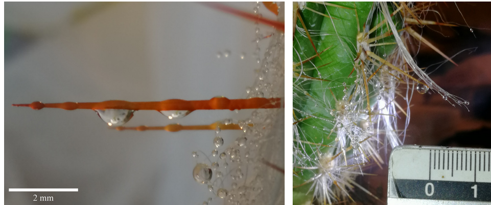
FIG. 21. (a) Cactus after 18 min and (b) 30 min of aerosol directed toward hairs and spines (The arrow points a large droplet an instant before sliding). The ruler is in the focal plane of the drop, and the black lines are 1 mm apart.
