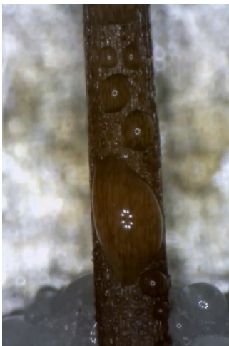
FIG. 7. Video of the top-view condensation experiment accelerated 64 times. In the first 16 seconds (higher magnification), there is the transition between regime I and II with the first distance coalescence events. Then, a few large droplets remain, and all the re-nucleated ones are continuously sucked into them (regime III). (Multimedia view: https://doi.org/10.1063/5.0066153.1 )
