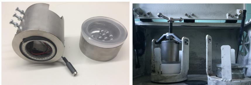
**Fig. 2.** Left, slot used for mounting the high speed camera directly on the jar equipped with a transparent lid. Right, the complete system mounted in the P4 planetary ball mill.
