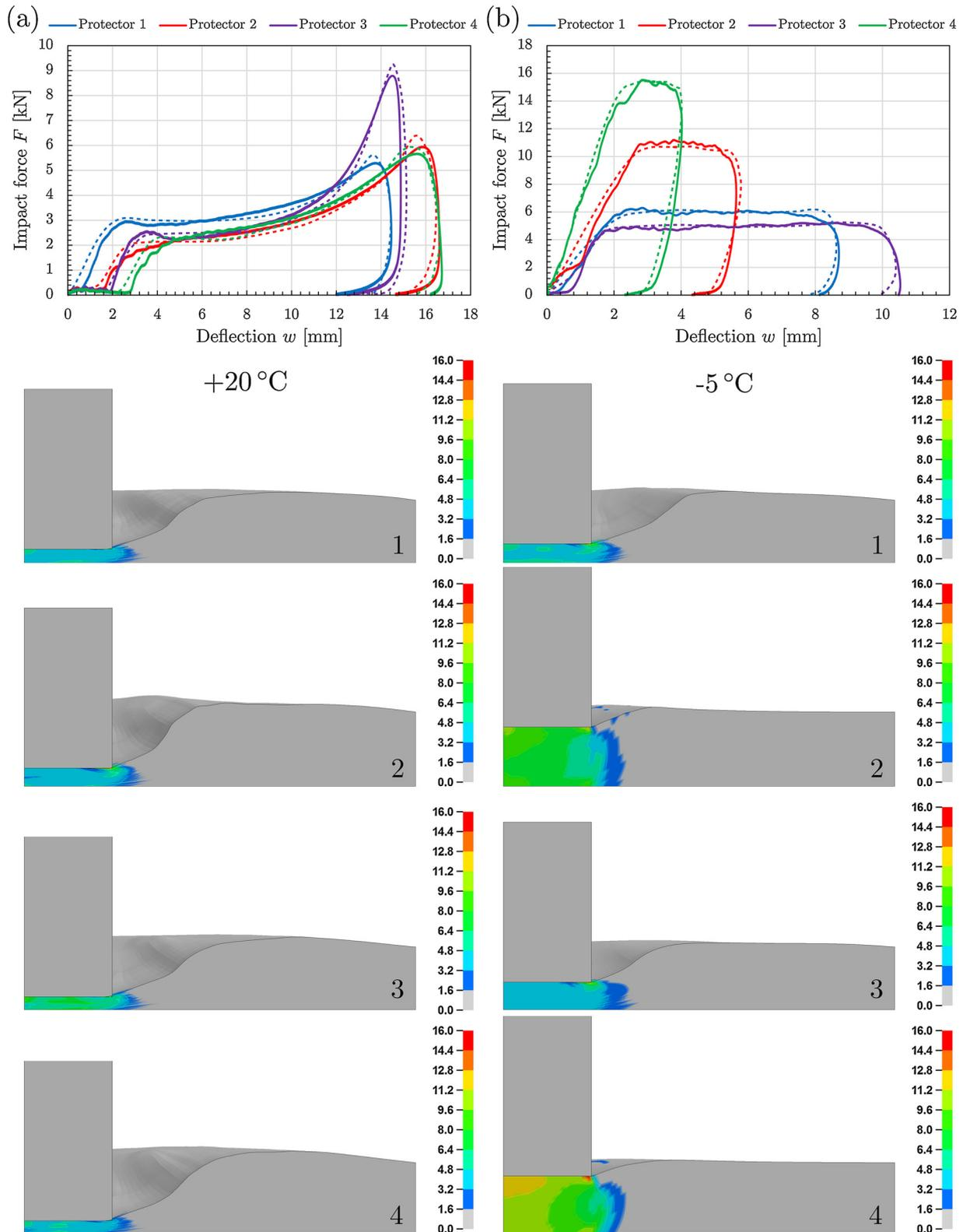
**Fig. 1.** Experimental (continuous) and FEM (dashed) force–deflection curves for the four tested protectors at (a) +20°C and (b) –5°C. In the bottom panels the snapshots from FEM simulations at the characteristic impact time ( $t = \tau$ , refer to values in Table 1) are depicted with contour plot of impact pressure (units in MPa). Stress field can be compared to the experimentally derived and analytically predicted stresses reported in Table 1.
