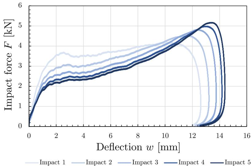
**Fig. 2.** Experimental force–deflection curves for protector 2 under multiple impact at +20 °C.
