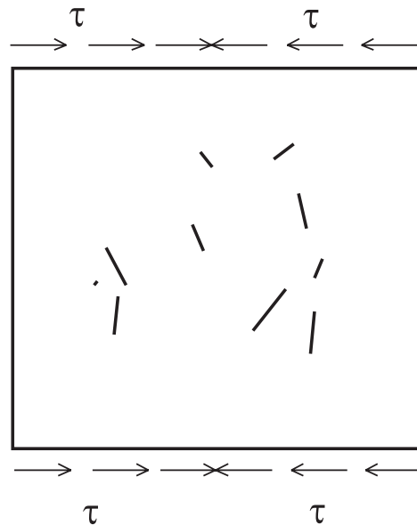
Fig. 7. Friction shearing stresses at the interfaces platens specimen.
