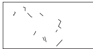
(B) intermediate crack distribution
