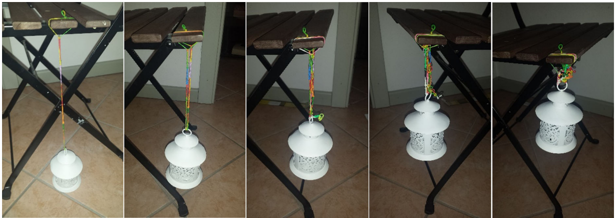
Fig. 4 Toy experiments inspired by the spider weight lifting. Elastic fibers are realized by a series of elastic bands and attached to a weight (candleholder). Four different experiments with different number of series and parallel elastic bands are
