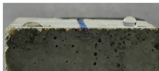
Figure 4. Water drops on a mortar sample: hydrophilic standard mortar surface (on the left side; contact angle roughly estimated to be about 45°) and hydrophobic mortar surface after treatment with a siloxanic hydrophobicizing agent in water solution (contact angle roughly estimated to be about 140°).
