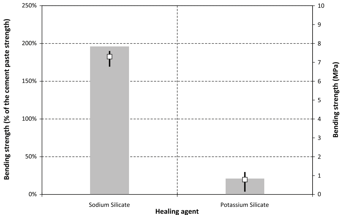
Figure 7. Preventive evaluation of sodium and potassium silicate as healing agents: white squares indicate the average bending strengths obtained on the samples reassembled using sodium or potassium silicate as a healing agent (values to be read on the right vertical axis); upper and lower edges of the solid black lines indicate, respectively, the maximum and the minimum values of the bending strengths obtained on the same samples (values to be read on the right vertical axis); gray bars indicate the average bending strengths obtained on the same samples as a percentage with respect to the initial cement paste strength (values to be read on the left vertical axis).
