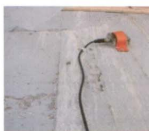
Fig. 3 : Cracks in the P_1 pier and the applied sensor (a). Relationship between signal detection distance and signal frequency (b).
