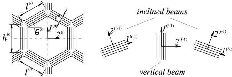
Fig. 4 Schematic of the honeycomb at level *i*.
