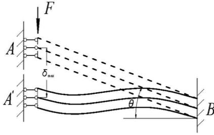
Fig. 1 SEM image of pure aspen wood [15]. Fig. 2 Hierarchical nano-honeycombs. Fig. 3 An inclined orthotropic beam.
