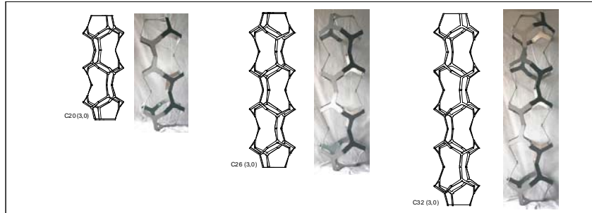
Fig. 10. Examples of nanotube with chiral index (3,0) and its practical realization.
