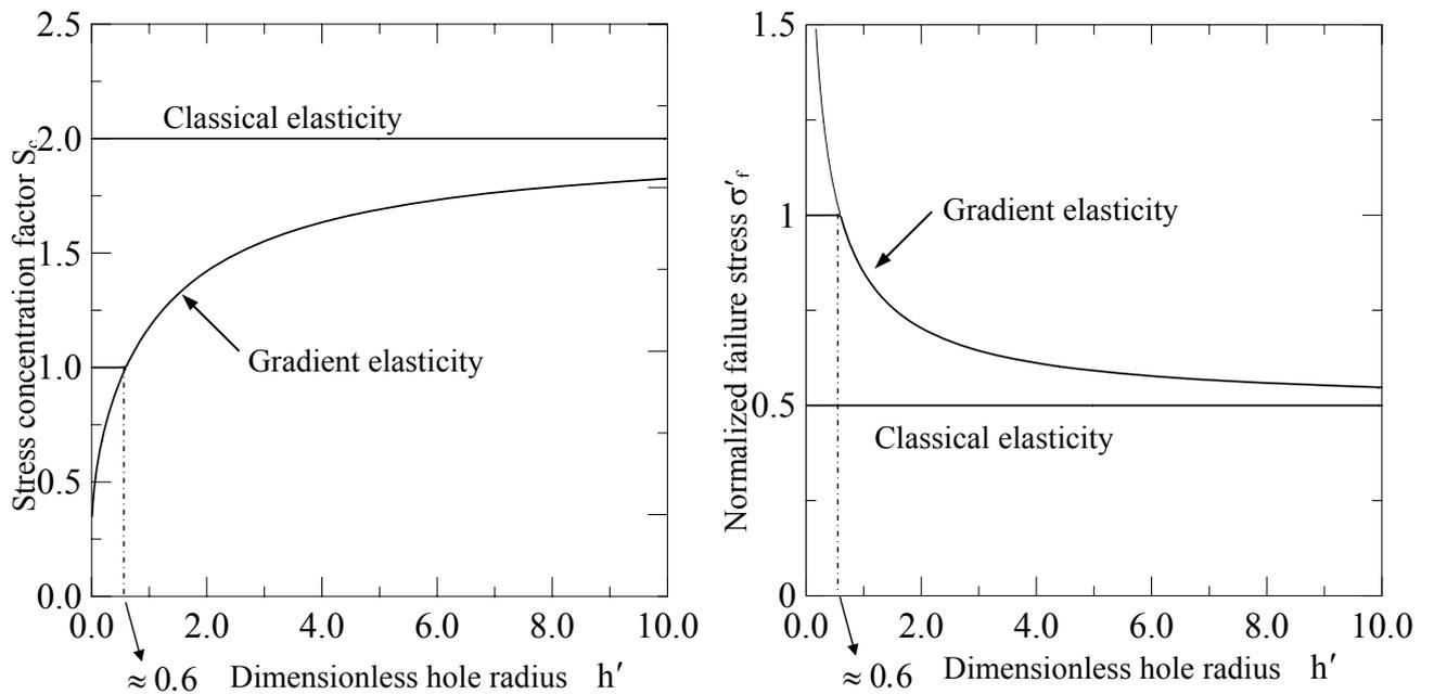
**Fig. 2:** Variation of (i) the stress concentration factor  $S_c$ , and (ii) the normalized failure stress  $\sigma'_f$  as a function of the dimensionless hole radius  $h'$ .
