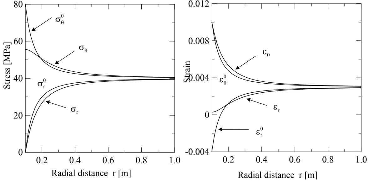
**Fig. 1:** Plots of (i) radial and tangential stresses, and (ii) radial and tangential strains, in classical (dotted lines) and gradient (solid lines) elasticity for  $\alpha=0.1\text{m}$ ,  $\sigma=40\text{MPa}$ ,  $\nu=0.4$ ,  $E=8\text{GPa}$ ,  $\sqrt{c'}=86\text{mm}$ ,  $h'=1.826$ .
