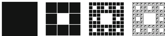
Fig. 2 The Sierpinski carpet ( D = 1.89 ) at different levels of observation; it corresponds to the cross section of a deterministic hierarchical bar in which the white zones represent the soft matrix and the black ones are the hard inclusions
